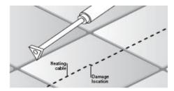
4. Once the grout is removed, carefully break away the tile using a hammer.
