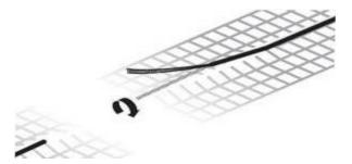
15. Heat only  $\frac{1}{2}$ " of the insulated end of the heating element to soften.
