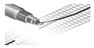
While the wire is still hot, use the wire strippers to remove 1/4" of the outer insulation to expose the heating element.
