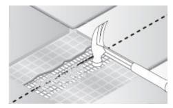
7. Remove sufficient mortar to expose 4-5 inches of heating cable on either side of the damage. Using scissors cut the tin foil from the cable to provide roomto install the splice.
