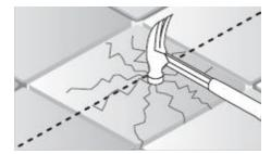
5. Remove any broken tile and vacuum other debris from the exposed surface to locate the damaged heating cable section.
