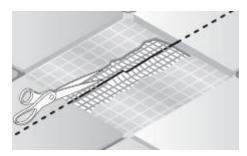
8. Remove at least 3 inches, and up to 5 inches of heating cable including the damaged section leaving two protruding ends of heating cable. If more than 5 inches of cable has been damaged, the mat must be replaced.
