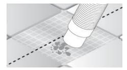
6. To expose the damaged section, break the mortar away from the heating cable with the ammer, making sure not to damage the cable.
