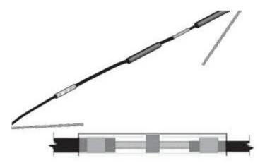
25. Centre the 4 black heat-shrinkable tubes over the installed splice connectors, and shrink in place using the heat gun.
