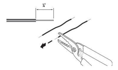
21. Slide splice connector onto one end of wire and crimp. Insert jumper wire into the splice connector and crimp.
