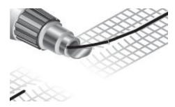
13. While the cable is still hot, use strippers to remove the outer jacket and foil layer to expose the heating elements.
