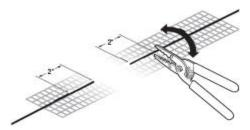
11. Flex the cable to break the insulation at the score.
