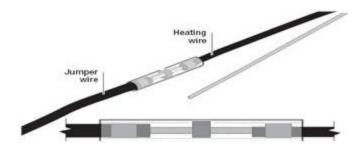
22. Slide two heat-shrinkable tubes onto each jumper wire.
