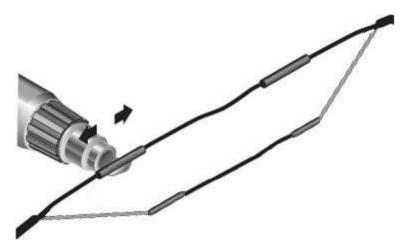
26. Slide the overall heat-shrinkable tubing with glue over the entire repair area and shrink in place using the heat gun.
