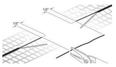
20. Strip 1/4" of insulation off both ends of each ju mper wire.
